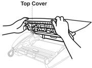
**3** Pull the jammed printout gently from the paper tray toward the *front* of the machine. If the printout is jammed, then pull it toward the *back* of the machine.
